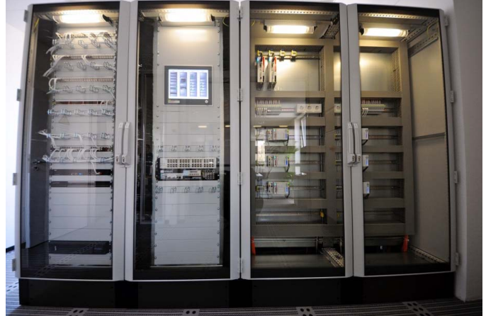
Figure 37: A setup with multiple IEDs connected to the DRTS/Co-Simulator in the SESA-Lab
