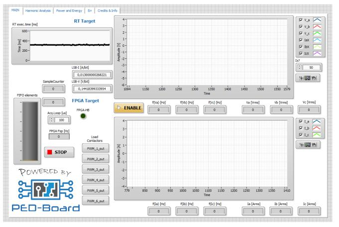
Figure 2. Front panel of the PED-Board based power quality analysis software.
