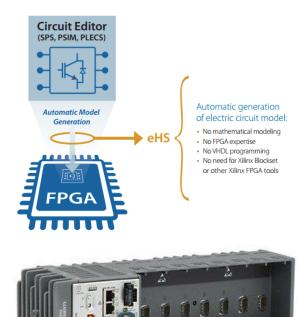
OPAL-RT eHS64 solver on NI cRIO-9039 Exchange of Real-Time digital data and analog signals ←→
