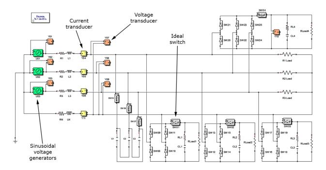
Figure 1. Simulink model for the electrical grid.
