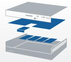
The OP4510 accepts any combination of four different I/O modules such as analog input, analog output, digital input and digital output.
